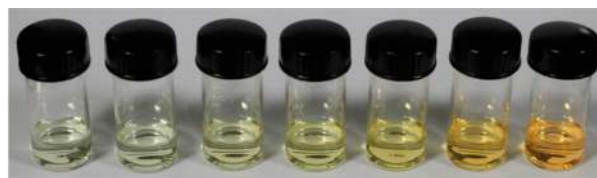
Figure 6. Photograph of (–)-1 ( 10^{-4} \text{ mol}\cdot\text{L}^{-1} ) in a mixed solution of MeOH and H 2 O in the ratios shown (under ambient light).
