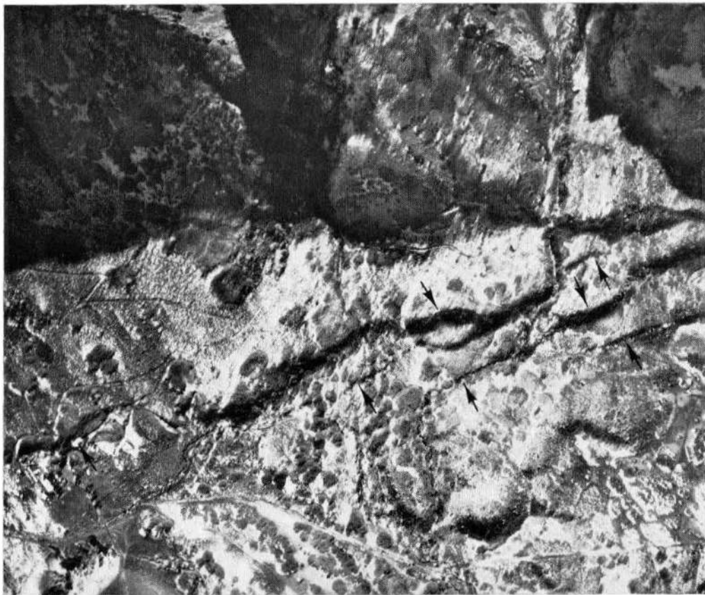
Fig. 39. A low-sun-angle photograph of the area included in the central square of Fig. 38, with the arrows in the same locations, showing how much more clearly the fault scarp can be seen (after Cluff and Slemmons, 1972)
