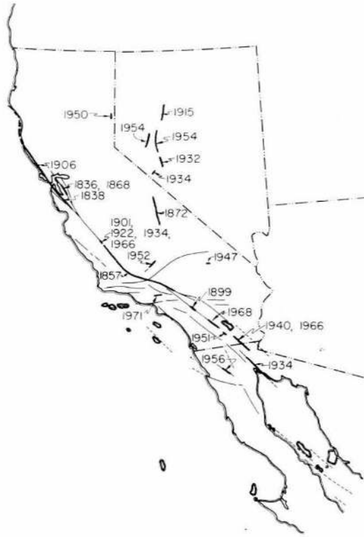
Fig. 27. San Andreas and associated fault zones in California, Nevada and northern Mexico. Zigzag lines show where surface of ground was broken during historic earthquakes and the dates of the breaks
