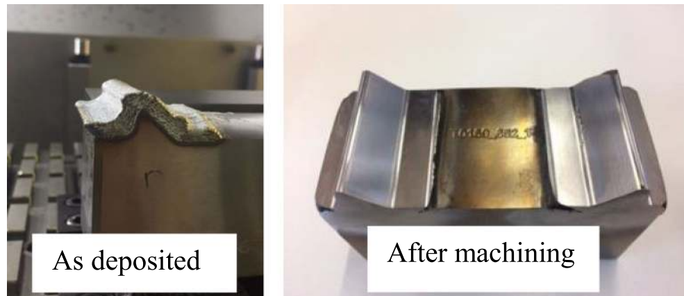
Fig. 13 Surface finish of samples in (a) as deposited and after machining states [62]
