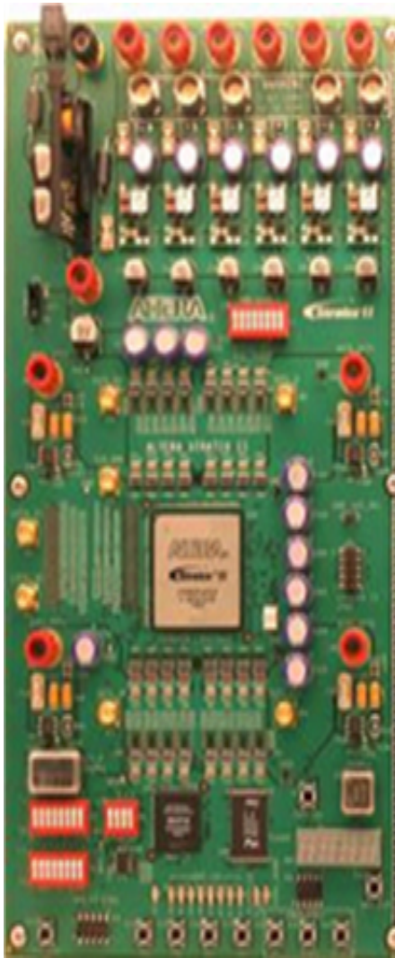
Fig. 9: Test platform for Stratix II EP2S60 power measurements
