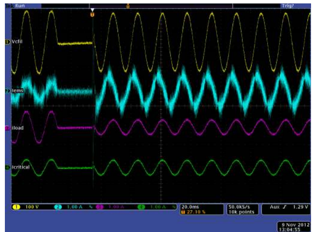
Figure 13. Experimental plots of main power source failure and EMS picking up the critical load.
