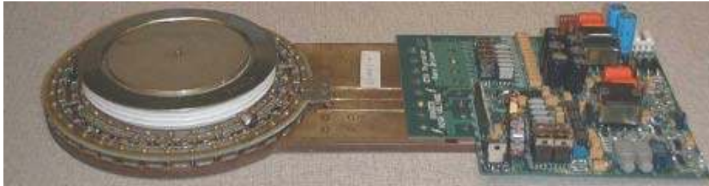
Fig. 4.10. 4000-A/4500-V ETO with the integrated gate driver [9].
