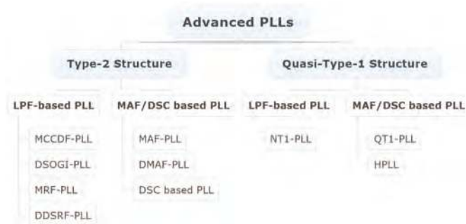
Figure 2. A general classification of typical advanced PLLs.
