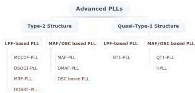
Figure 2. A general classification of typical advanced PLLs.
