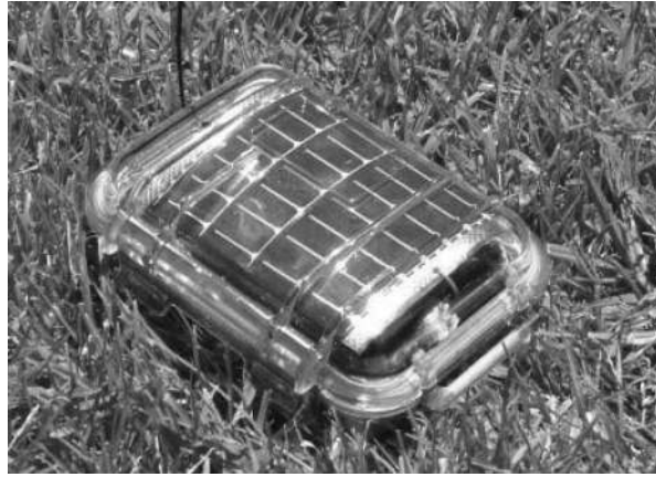
Fig. 4. Heliomote: an energy-harvesting sensor node, which provides environmental energy tracking capabilities.
