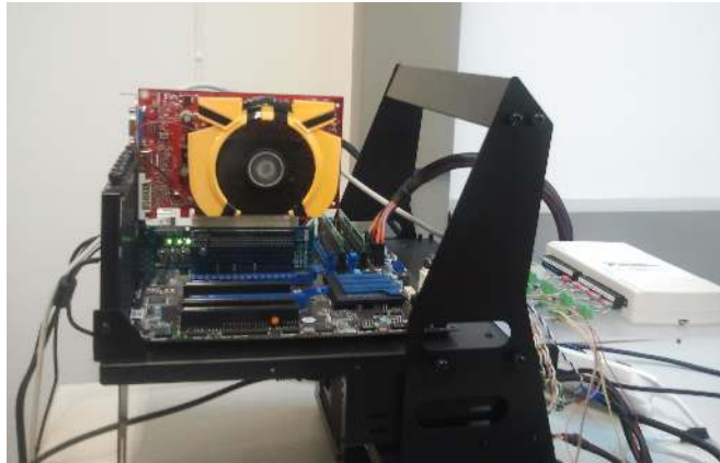
Figure 4.7: Power measurement testbed with GT240 graphics card [99]. © 2013 IEEE
