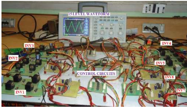
FIGURE 15. Experimental setup for fifteen level inverter with VR.
