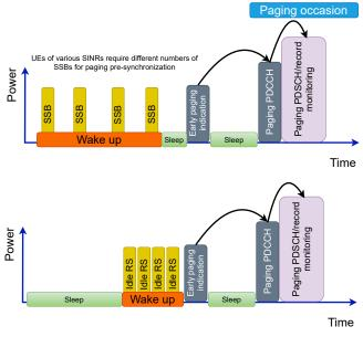
Fig. 5. Idle/inactive mode assisting reference signal.
