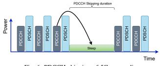
Fig. 6. PDCCH skipping of 5G new radio.
