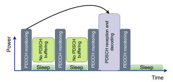
Fig. 3. Cross-slot scheduling and resource allocation.
