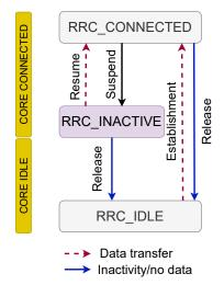
Fig. 1. RRC state transition in 5G new radio.
