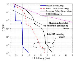
Fig. 7. Downlink outage latency: impact of scheduling delay.
