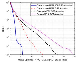
Fig. 9. Wake up time: impact of 5G NR paging procedures.
