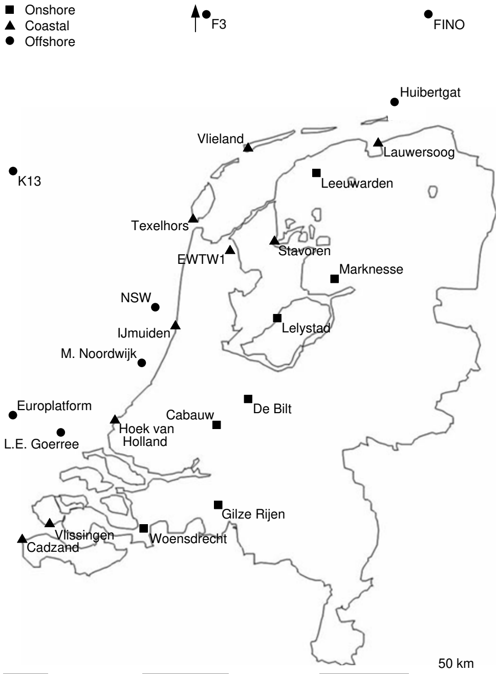
Figure A.1: Inland, coastal and offshore wind speed measurement and numerical weather prediction locations.
