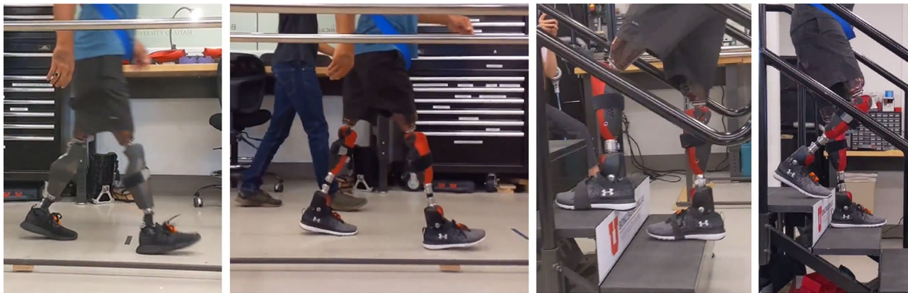
Figure 4. The passive and powered prostheses donned by the participant. From left to right, the images show the participant walking with his prescribed prostheses, walking with the powered prostheses, ascending stairs step-over-step with the powered prostheses, and descending stairs with the powered prostheses. For all conditions the participant was wearing Xsens Motion Tracking IMUS on the prostheses.
