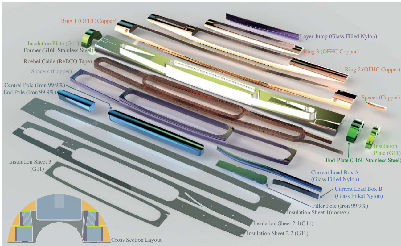
Figure 4. Rendering showing an exploded view of all the parts making up one of the Feather-M2 magnet poles. Visible from top to bottom are the copper rings, the spacers, the coil-windings and joint area, the former, the iron poles and the G11 insulation sheets.
