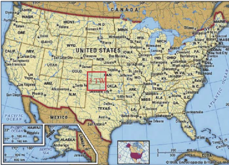
Figure 5. The red square shows the amount of land needed for a solar energy farm operating at 10% efficiency to match the 3 TW of power currently consumed in the United States.
