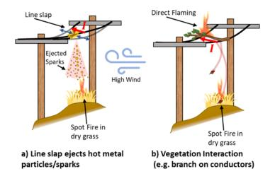
Figure 2: A schematic illustration of ignition caused by powerline failure. The two main mechanisms are interactions between conductors (a) and interactions of vegetation and conductors (b).
