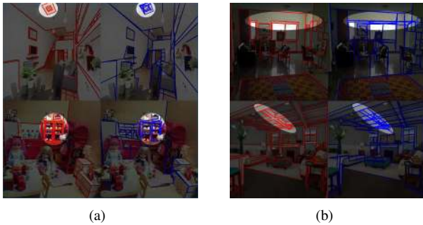
Figure 6. Failure cases: (a) image samples that contain small rectangulars; (b) image samples that contain very close co-linear line segments.
