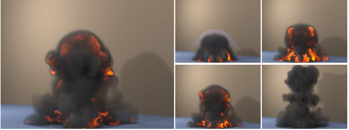
Figure 3: A charge is detonated within a small four-walled chamber at t = 0 . Shown on the left is a smoke plume at t = 0.04s , and on the right its development, at times .005s , .02s , .03s and .115s . This was solved on a 200 \times 300 \times 200 grid.
