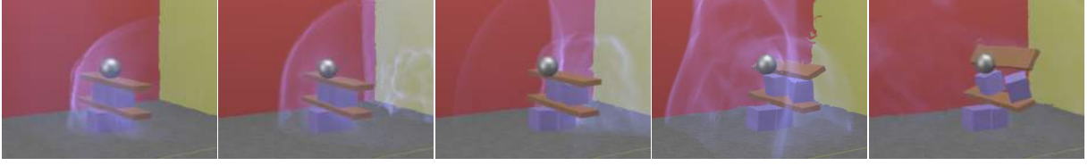
Figure 2: A planar shock enters an enclosed domain and disrupts a stack of rigid bodies. It reflects off of the back wall, hits the stack of objects again, and exits the domain. Times .0011s, .0018s, .003s, .0043s and .0053s are shown. The grid size is 225 \times 150 \times 150 .
