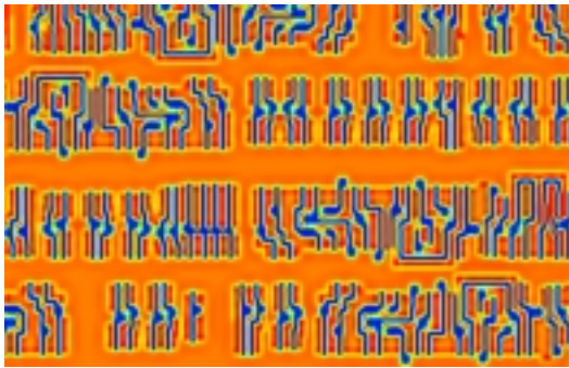
Figure 4: Simulation result of multiple interactions among standard-cells between adjacent rows and within each row
