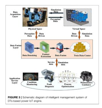
the Digital Twins (DTs) technology is applied to it. The specific DTs-based power IoT system is shown in **Figure 3**.
