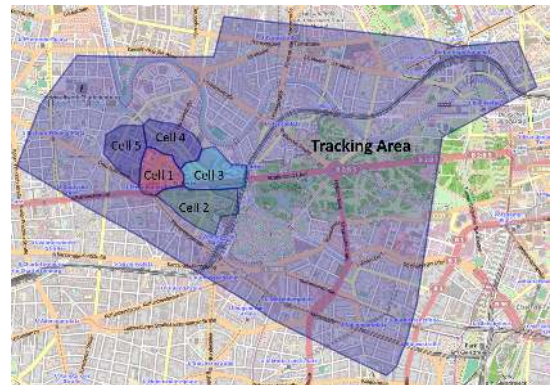
Fig. 5. LTE tracking area and cells of a major operator in a city
