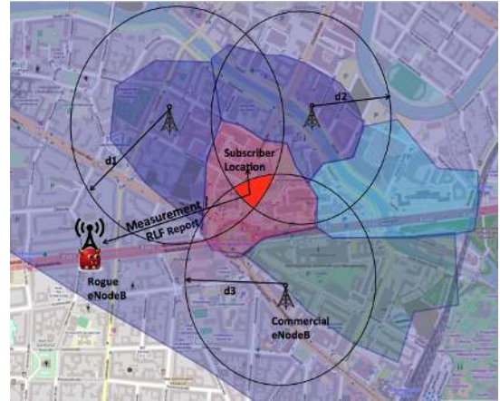
Fig. 7. Determining subscriber's precise location using trilateration (L3)
