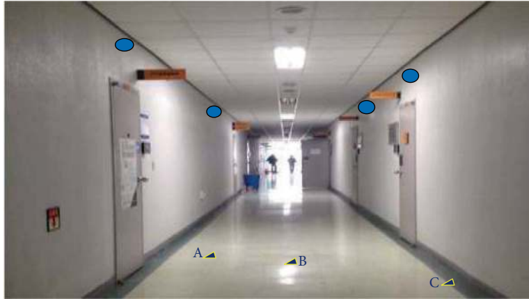
FIGURE 10: Experimental environment: beacons deployed in the corridor where blue circular dots along the wall of the corridor represent beacon deployment positions, and measurement places are marked on the floor as A, B, and C.
