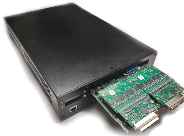
Figure 30. Setup of 2 FMC-ADC-TDC modules (green electronic boards) mounted on AFCK board inside mTCA Chassis (black box). AFCK and modules are temporarily ejected for presentation/maintenance purposes.
