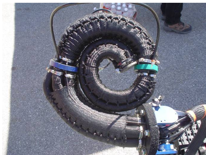
Fig. 1. OctArm V - Continuum manipulator
