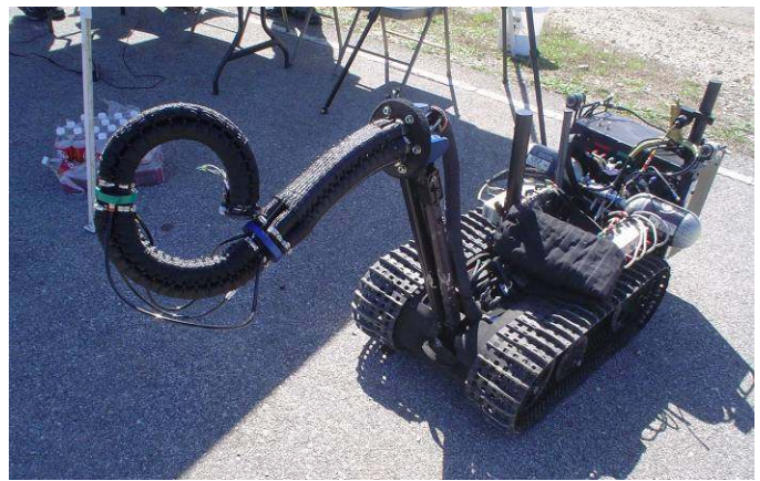
Fig. 7. OctArm V mounted on Foster-Miller TALON system.
