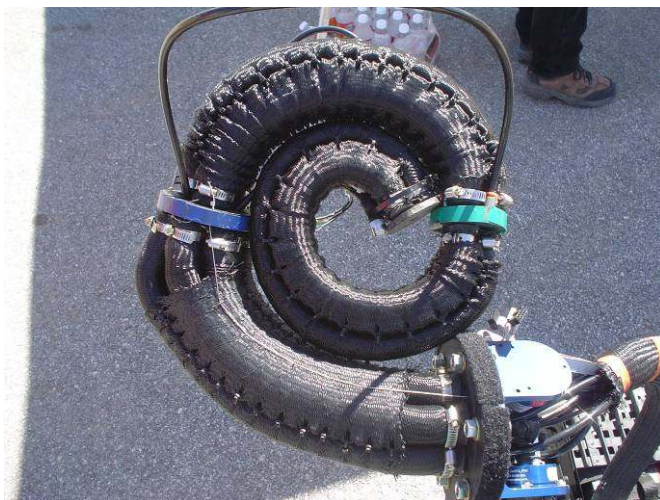
Fig. 1. OctArm V - Continuum manipulator
