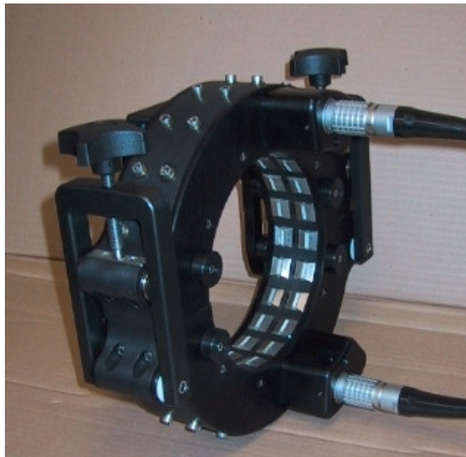
FIGURE 4. Solid transducer assembly for 8 inch pipe showing array of dry coupled piezoelectric transducers.
