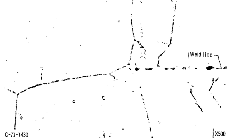
(b) Auto-vac cleaned at 1200° C for 1 hour prior to solid-state welding at 980° C.
