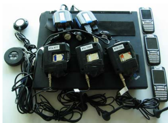
Figure 1. Our GSM/WiFi data collection device: one WiFi card, two GPS units (left), and three Sony Ericsson GM28 GSM modems (center) are connected to an IBM Thinkpad T30 laptop. The modems require external antennas (bottom) and we have modified them to be powered via USB hubs. Three Audiovox SMT5600 phones, one for each network provider, are shown on the right,
