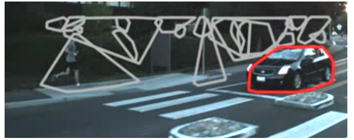
Fig. 3: Segmentation and tracking failures are the most common source of object recognition errors. In this example, a pedestrian gets segmented together with a large stretch of curb, resulting in a false negative, while a well-segmented car is correctly identified. Best viewed in color.
