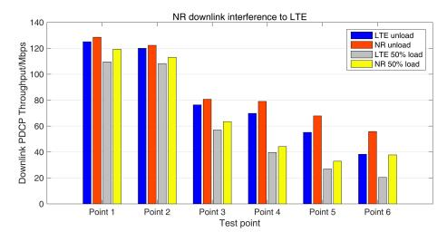
5.2.2. LTE Downlink Interference from NR of Adjacent Cells to DSS Test Cells The test results are shown in Figure 15.
