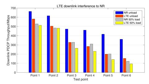
Figure 14. LTE to NR downlink interference test results.
