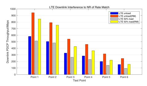
Figure 20. LTE to NR Downlink Interference Test Results after Rate Matching.
