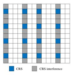
Figure 6. Schematic diagram of DSS interference.
