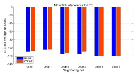
Figure 16. NR terminal to LTE uplink interference test results.
