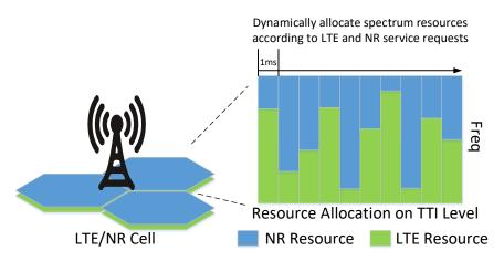
Figure 2. DSS dynamically adjusts spectrum resources.
