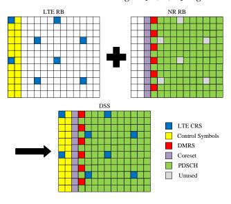
Figure 9. Schematic diagram of rate matching.
