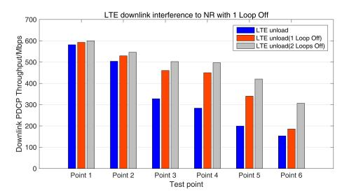
Figure 18. LTE to NR downlink interference test results—buffer setting (no load).
