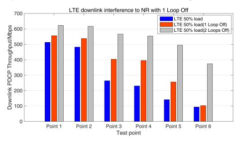
Figure 19. LTE to NR downlink interference test results—buffer setting (50% load).
