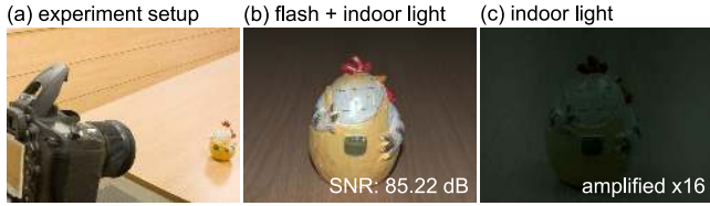
Fig. 7. (a) Capture setup using a DLSR camera. (b) Captured image using the flash light (1/250 sec., f/16 , ISO 100). Its high SNR of 85.22 dB, confirms that the built-in flash is bright enough to avoid the need for a darkroom. (c) Captured image (amplified \times 16 for visualization) with only ambient illumination without flash using the same settings.
