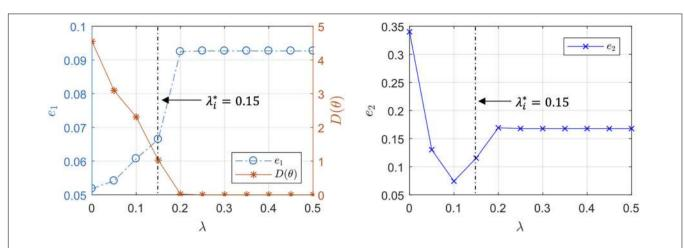
**FIGURE 5** | Representative trends of the output prediction error  $e_1$ , the internal state prediction error  $e_2$ , and the parametric deviation distance in a subject with respect to the regularization weight  $\lambda$ .
