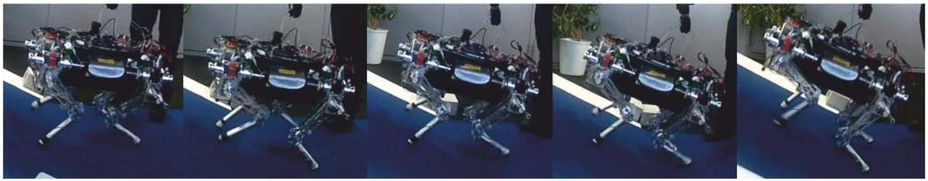
Fig. 6. StarLETH transits from flat to sloped terrain with 21^\circ (38%) while trotting (adapted from [16])
