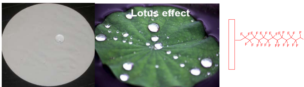
Figure 12. High contact angle and the non-wetting of porous PEEK membrane surface (ethanol liquid drop)
