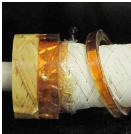
Figure 22. Broken tubesheet due to high differential pressure.
