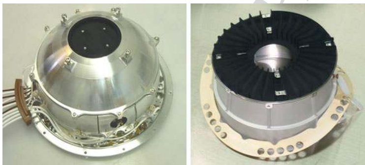
1979 Fig. 41 Copper sulfide blackened energy analyzer (left) and entrance section (right)
