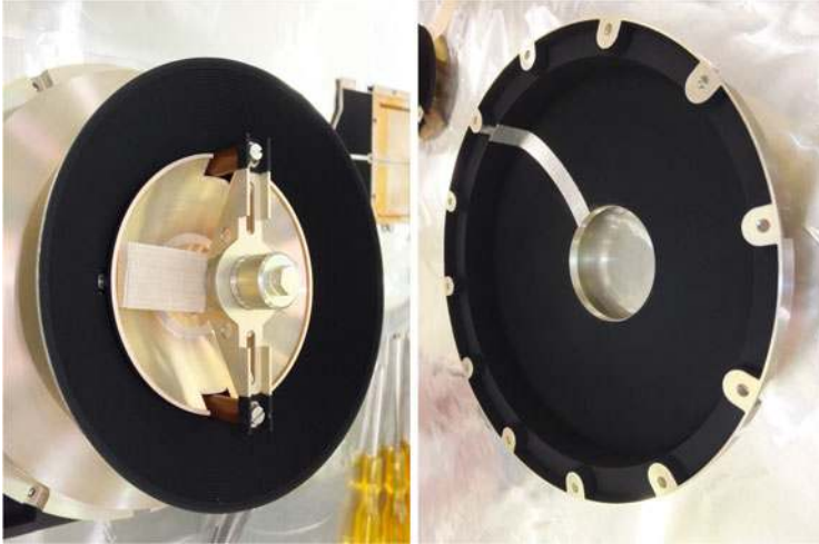
Fig. 62 HEP-ion collimator (left) and electrostatic mirror (right) of the TOF unit blackened with conductive paint
