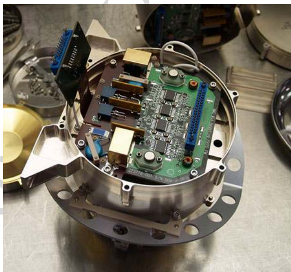
Fig. 28 Negative high voltage board installed in the chassis of MIA. A Hypertac connector from ASIC on the MCP anode is also shown
