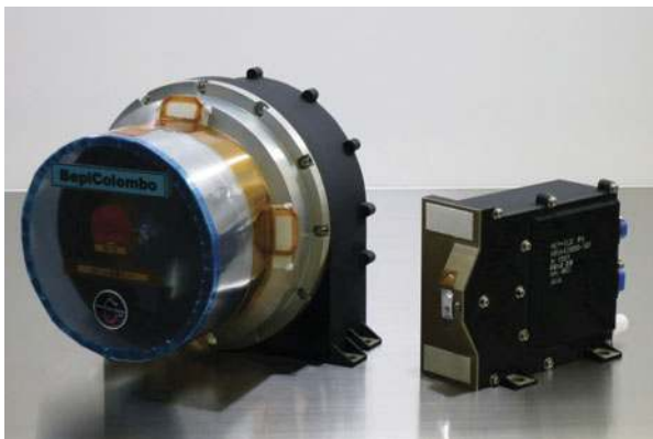
2601 Fig. 53 HEP-ele and HEP-ion 2602 with some non-flight items (blue) 2603 in a clean bench 2604
