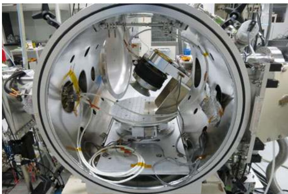
Fig. 67 HEP-ion set on the multi-axial turntable system in the vacuum chamber at the beamline calibration facility
