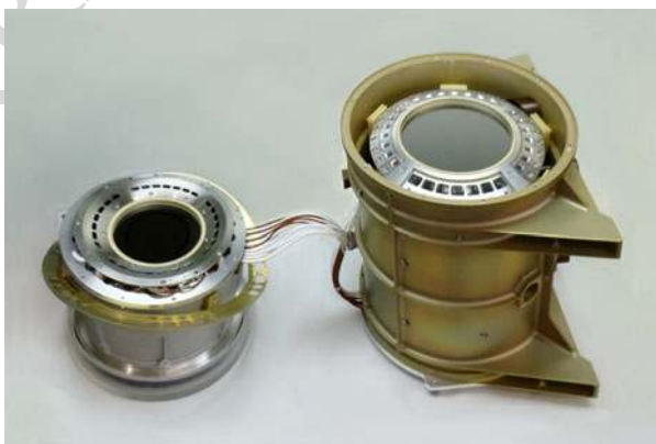
1979 Fig. 41 Copper sulfide blackened energy analyzer (left) and entrance section (right)
