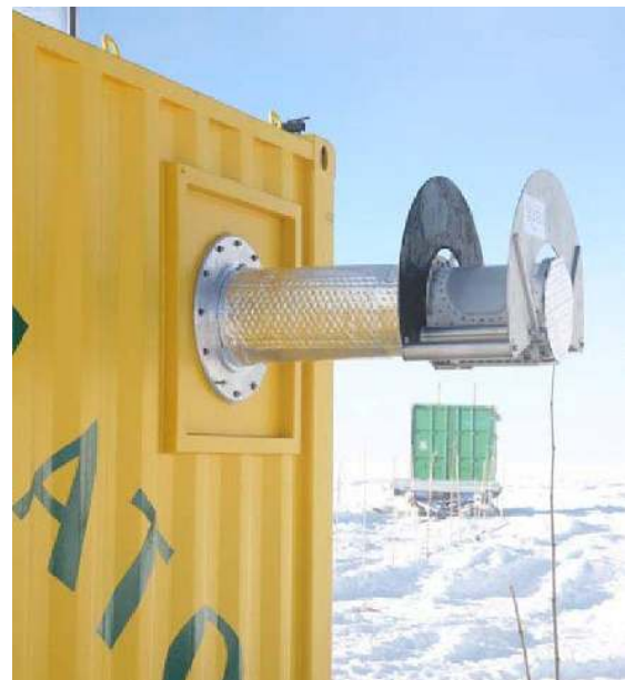
Figure 4b: The Pre-HEAT telescope installed onto the PLATO instrument module at Dome A. Photo from January 2008, courtesy Z. Zhu and Z. Xu.
