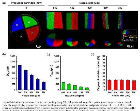
(b) Measurement of hydraulic diameters of the single strut ( $D_{H,S}$ ) and a quarter of a strut ( $D_{H,Q}$ ), i.e., one compartment. (c) Degree of miniaturization, the percentage ratio of  $D_{H,S}$  to  $D_{H,Q}$ , which indicates the ratio of the miniaturized hydraulic diameter of the printed strut from the whole to each compartment.
