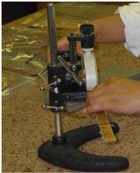
Figure 4.11 Durometer hardness testing.
