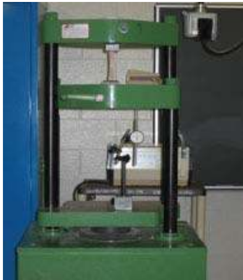
Figure 4.8 Tensile strength test of a composite sample using the Instron Universal testing machine.
