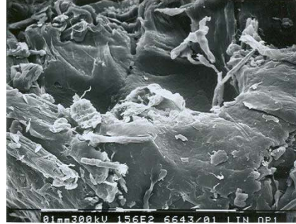
b) Silane treated flax in composites
