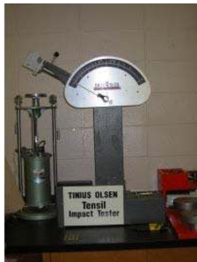
Figure 4.9 Tensile-impact strength tester.
