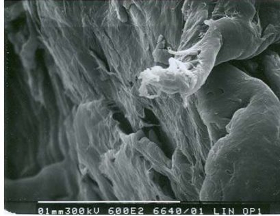
a) Untreated flax in composites
