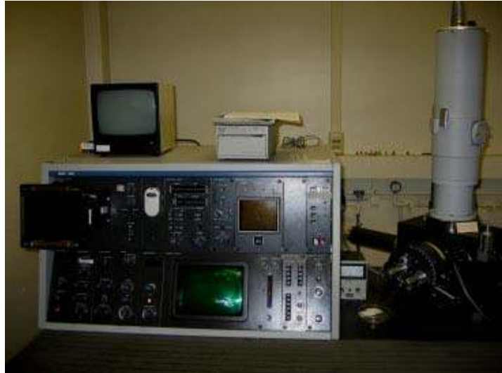
Figure 4.5 Scanning electron microscope.
