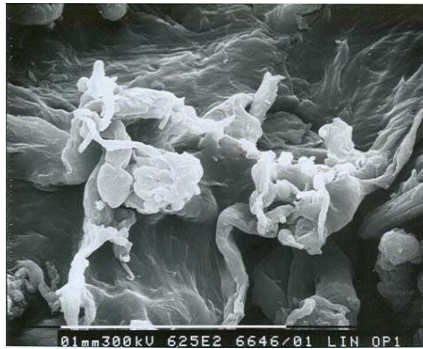
c) Benzoylation treated flax in composites
