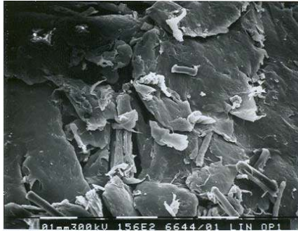
a) Untreated flax in composites
