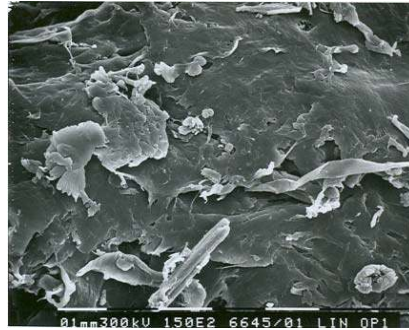
b) Silane treated flax in composites
