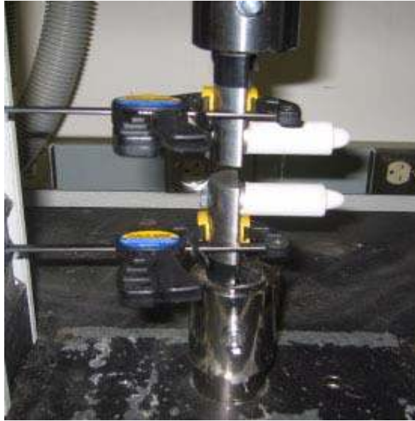
Figure 4.6 Set up for the tensile strength of fiber bundle.
