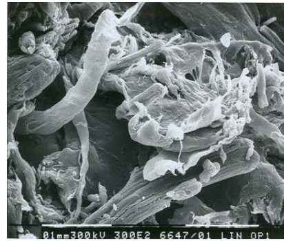
d) Peroxide treated flax in composites
