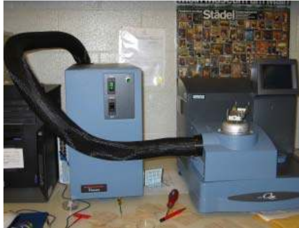
Figure 4.13 DSC melting point test of composites.
