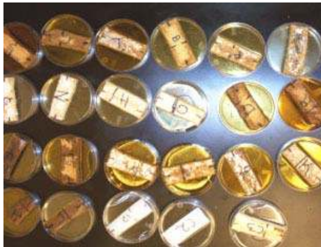
Figure 4.12 Water absorption test of composites.
