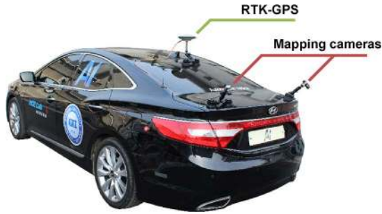
Fig. 4. Mapping system equipped with centimeter-level accuracy RTK-GPS and two down-looking camera is used to capture the road surface image.
