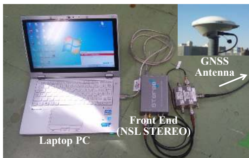
Figure 4. Set-up of software GNSS receiver.
