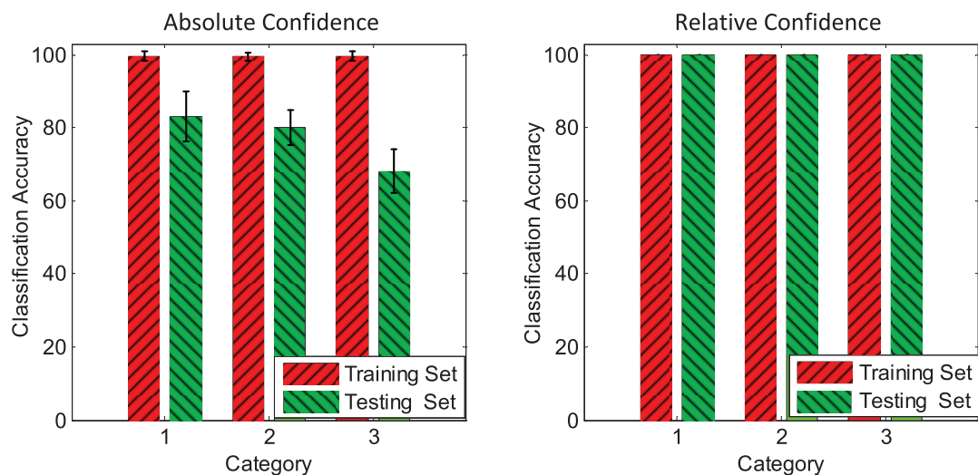
Figure 12. The average accuracies for the classification of spatiotemporal patterns. There are 3 categories to be classified. The average accuracies are represented by shaded bars. Two types of criteria for making decision are proposed and investigated. The left is the absolute confidence criterion, and the right is the relative confidence criterion. All the data are averaged over 100 runs. doi:10.1371/journal.pone.0078318.g012
