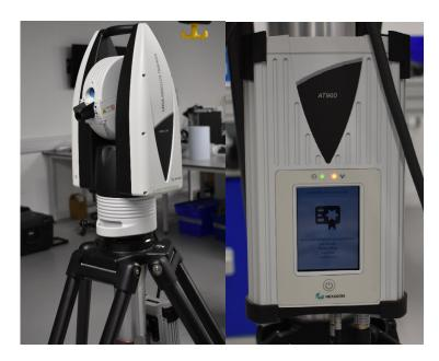
Figure 6. Laser tracker and its controller.
