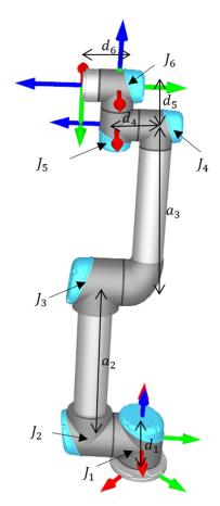
**Figure 2.** Typical industrial robot (UR5) schematics ( $d_i$ , i = 1, 4, 5, 6 and  $a_i$ , i = 2, 3 parameters refer to the DH parameters of the UR5).
