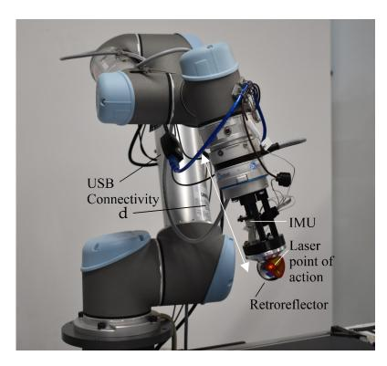
**Figure 5.** UR5 with a retroreflector mounted on it as the target for the laser tracker.
