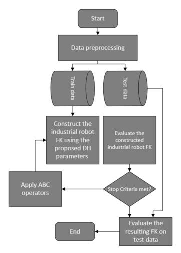
Figure 1. Overall calibration flowchart.
