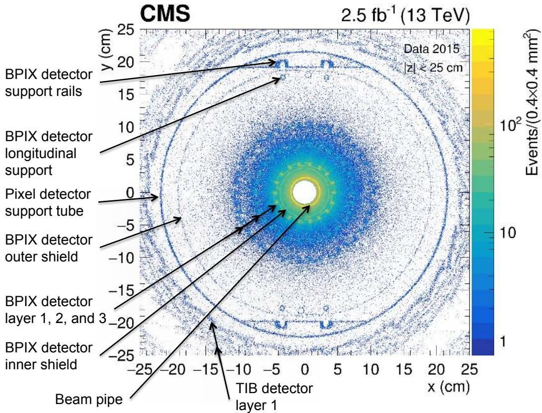
**Figure 4.** Hadrography of the tracking system in the  $x$ - $y$  plane in the barrel region ( $|z| < 25$  cm). The density of NI vertices is indicated by the color scale. The signatures of the beam pipe, the BPIX detector with its support, and the first layer of the TIB detector can be observed above the background of misreconstructed NIs.
