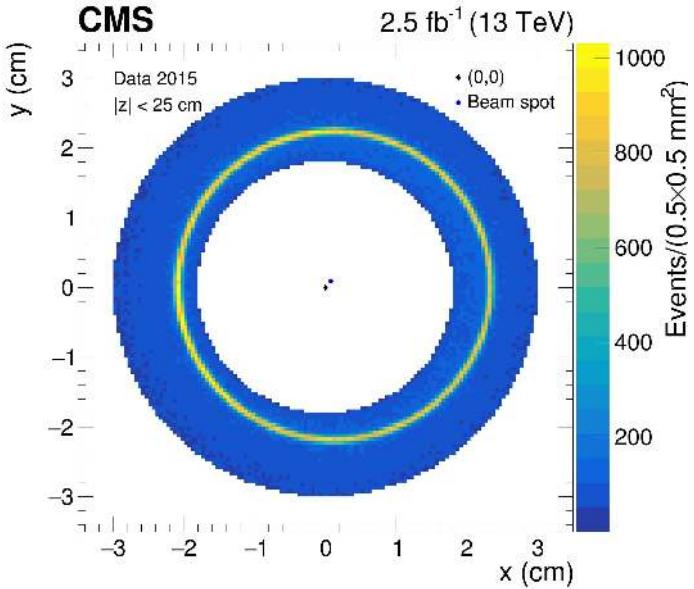
**Figure 5.** The beam pipe region viewed in the  $x$ - $y$  plane for  $|z| < 25$  cm before background subtraction. The density of NI vertices is indicated by the color scale.  $(0, 0)$  is the origin of the CMS offline coordinate system, which is discussed in section 7.1. The blue point in the center of the distribution corresponds to the average beam spot position of  $x_{\text{bs}} = 0.8$  mm and  $y_{\text{bs}} = 0.9$  mm in 2015.
