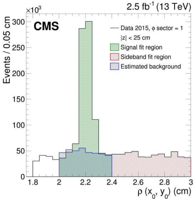
**Figure 6.** The density of NI vertices versus  $\rho(x_0, y_0)$  for a  $\phi$  slice of the beam pipe located near  $\phi = 0$  (black line) for  $|z| < 25$  cm before background subtraction. The green hatched area corresponds to the signal region, the red hatched area corresponds to the sideband region used to fit the background, and the blue hatched area corresponds to the estimated background in the signal region.
