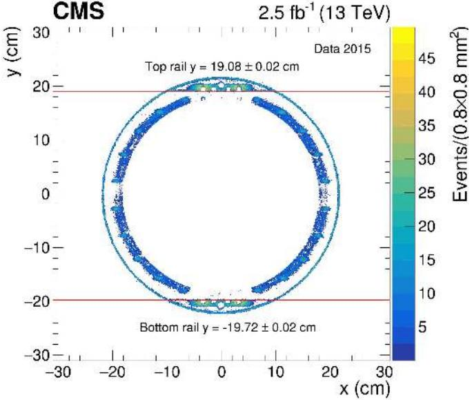
**Figure 12.** The BPIX detector support rails after background subtraction in the  $x$ - $y$  plane for the combined tracking detector barrel and endcap regions. Horizontal red lines correspond to the fit of the BPIX detector support rails. The density of NI vertices is indicated by the color scale.
