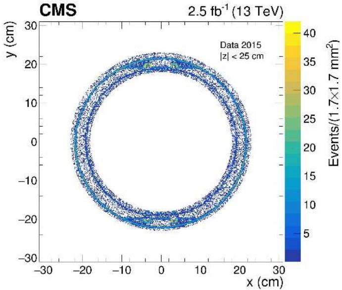
**Figure 10.** The region of the pixel detector support tube viewed in the  $x$ - $y$  plane for  $|z| < 25$  cm before background subtraction and removal of the  $\phi$  regions with additional structures. The density of NI vertices is indicated by the color scale. Two circular structures are visible. The circle with the smaller radius corresponds to the BPIX detector outer shield, while the one with the larger radius is the pixel detector support tube (also visible in figure 4).
