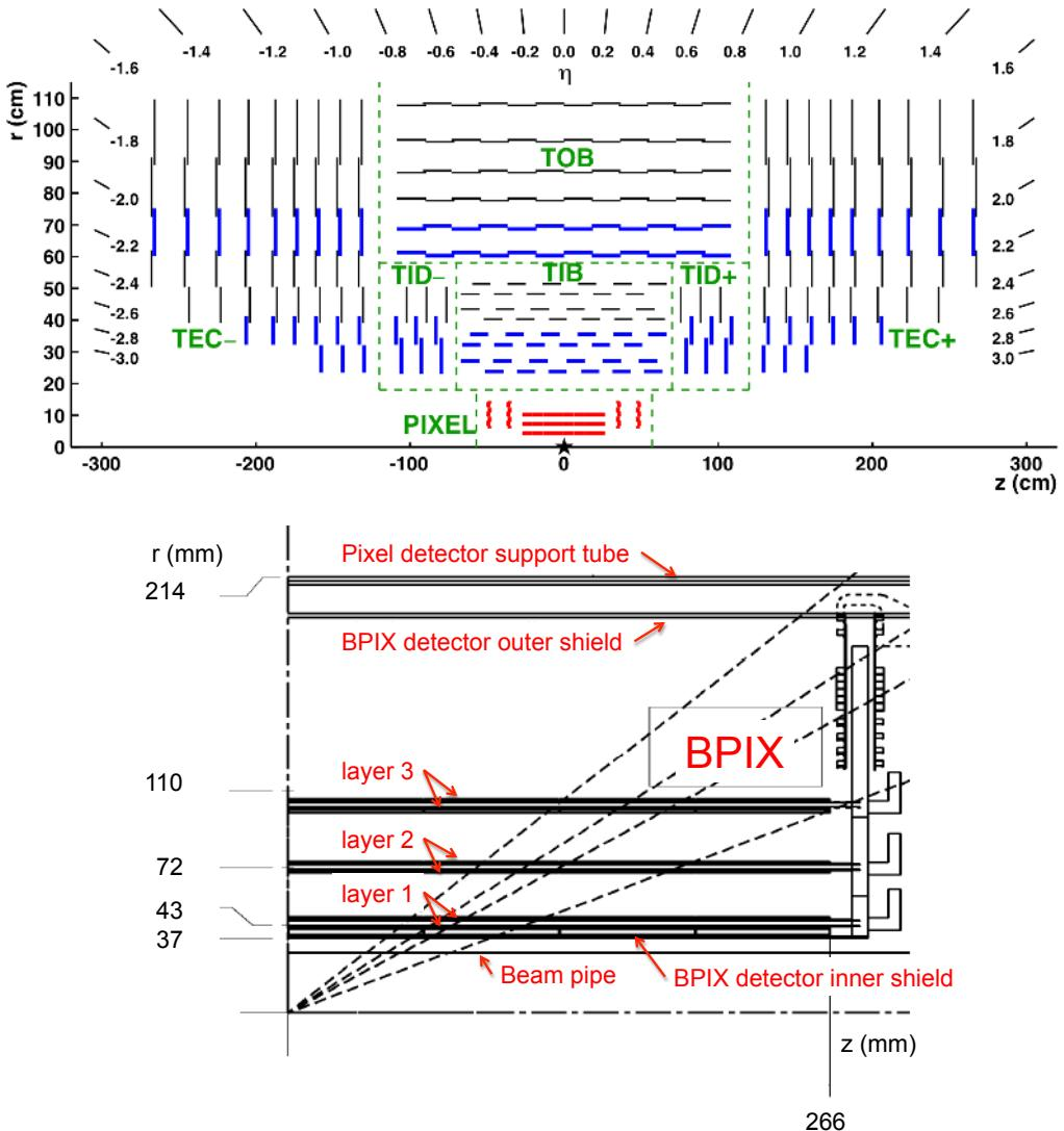
**Figure 1.** (Upper) Schematic view of the CMS tracking detector [1], and (lower) closeup view of the region around the original BPIX detector with labels identifying pixel detector support tube, BPIX detector outer and inner shields, three BPIX detector layers, and beam pipe.
