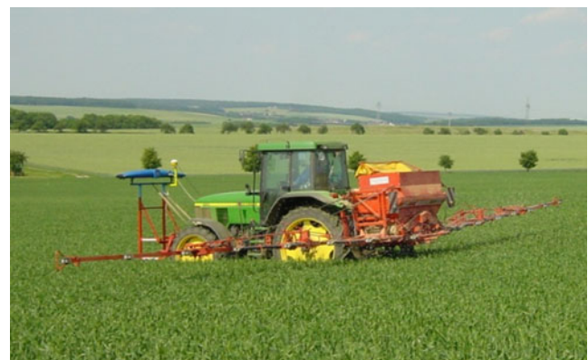
Fig. 3 Implementation of variable-rate technology for site-specific nitrogen application in a winter wheat field in southern Germany (From: Schmidhalter U., Life and Food Sciences Center Weihenstephan of the Technische Universität München)
