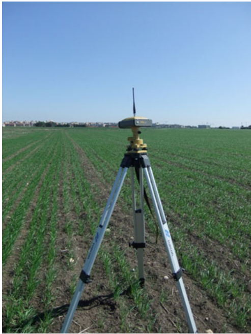
Fig. 1 Sampling location (point coordinates) and elevation can be recorded by using a differential global positioning system (DGPS, HiPer® 27 Pro, TOPCON). It enhances the quality of location data gathered using global positioning system (GPS) receiver. The figure shows base station of the instrument positioned in a wheat field
