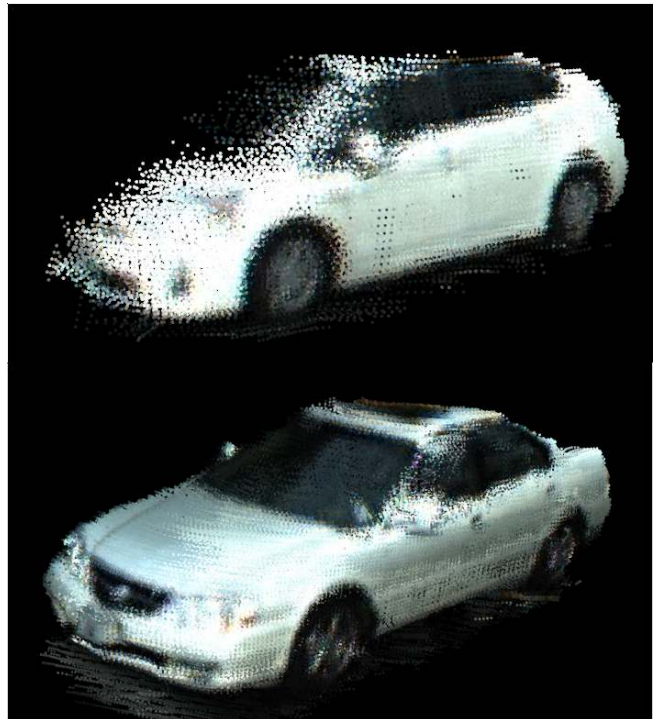
Fig. 1. Two 3D car models created using the color-assisted grid search alignment method. Note that these cars were moving while the alignment was being performed.
