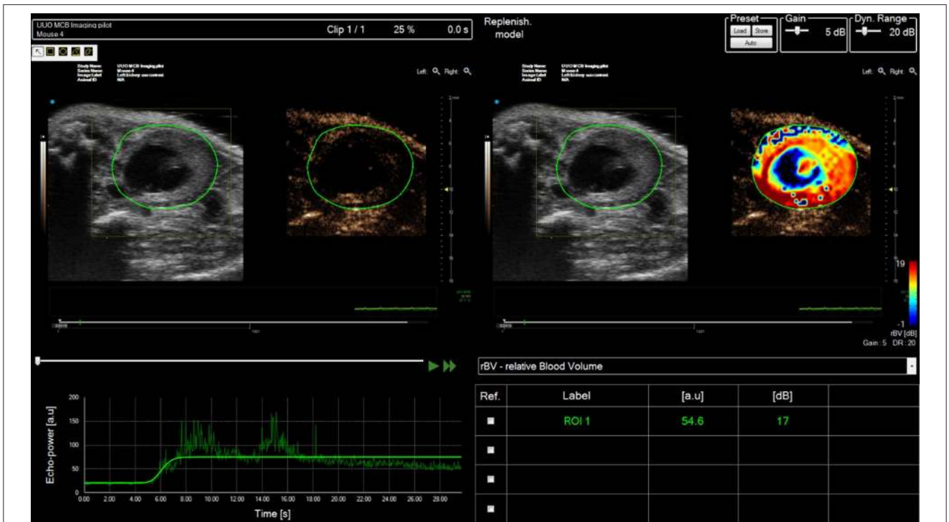
FIGURE 9 | Contrast analysis of data-set acquired from right mouse kidney post ischemia-reperfusion (IRI) injury after tail-vein bolus injection of SonoVue. Mouse scanned in prone position. Multiple regions of interest (ROIs) can be drawn onto the image and the enhancement can be tracked as a function of time (bottom LHS). The relative enhancement of each ROI relative to pre-contrast image can be calculated and color-encoded (Top RHS).
