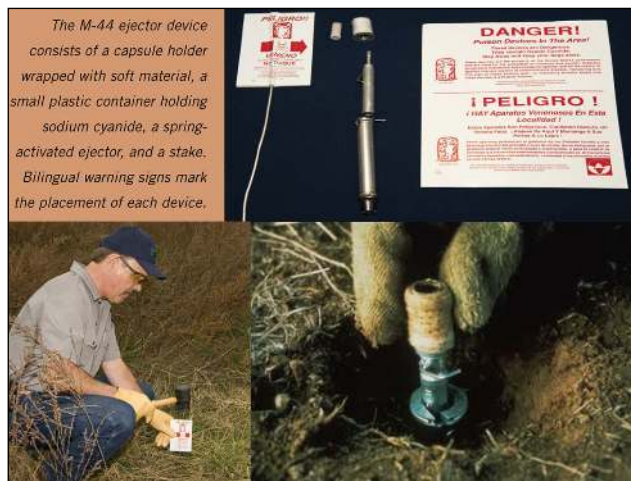
Figure 2. M-44 explosive poison (sodium cyanide) delivery device for killing wildlife (Factsheet May 2010, US Department of Agriculture Wildlife Services; http://1.usa.gov/281v69N ).
