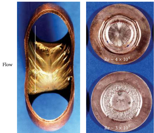
FIGURE 8: Typical copper specimens after testing in single phase flow. (a) Reducer (39 to 25.6 mm), Re \ 2.8 \times 10^5 in larger tube ([40]). (b) 180°, 2.5 D bend at Re of 70000 ([37]). (c) Impinging specimens at 9.5 mm from 9.5 mm diameter jet ([40]).
