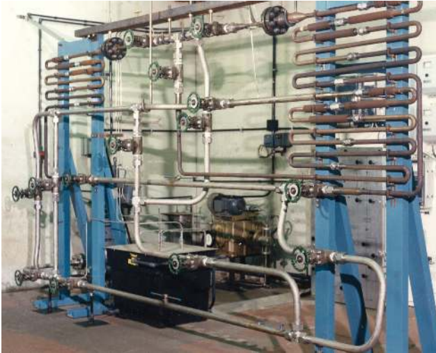
FIGURE 24: High pressure and high temperature flow loop for FAC studies on British AGR components.
