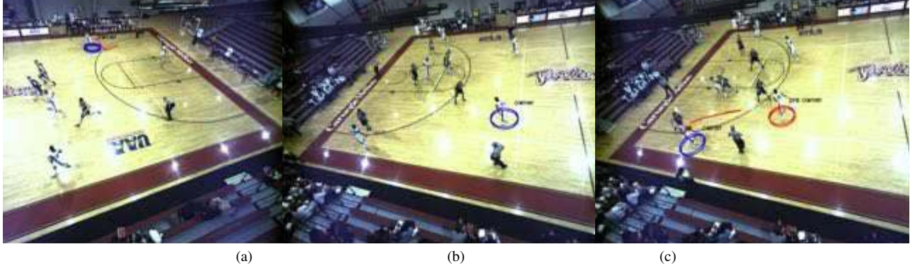
Figure 10. Examples where the ball is visible and occluded (both fully and partial): (a) In the far corner the resolution is low, and the background is of a similar color to the ball, (b) The ball is occluded by the player, (c) A pass is clearly visible.
